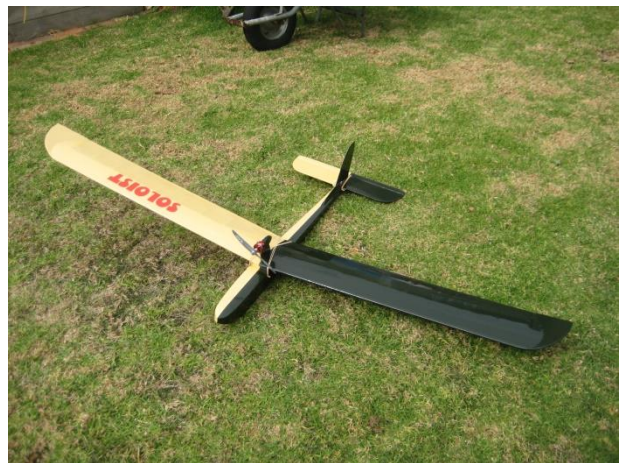
Dayle Montgomery's 72" E-Max powered Soloist, a glider, weight 21.6 oz (613 grams). FC 28-05 2840 Kv outrunner, 18 amp esc, 6 x 4 prop, 1000 mAh 2s Li-po giving about 410 grams of thrust, wing loading of 6.17 oz/square foot. T
