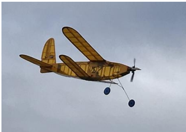
Dayle Montgomery's 1938 J.E. Leadbetter designed Dragonfly. 28" top wing and a 20" lower wing. It was previously rubber powered but now sports 2s electric and a linear servo for rudder only control.
